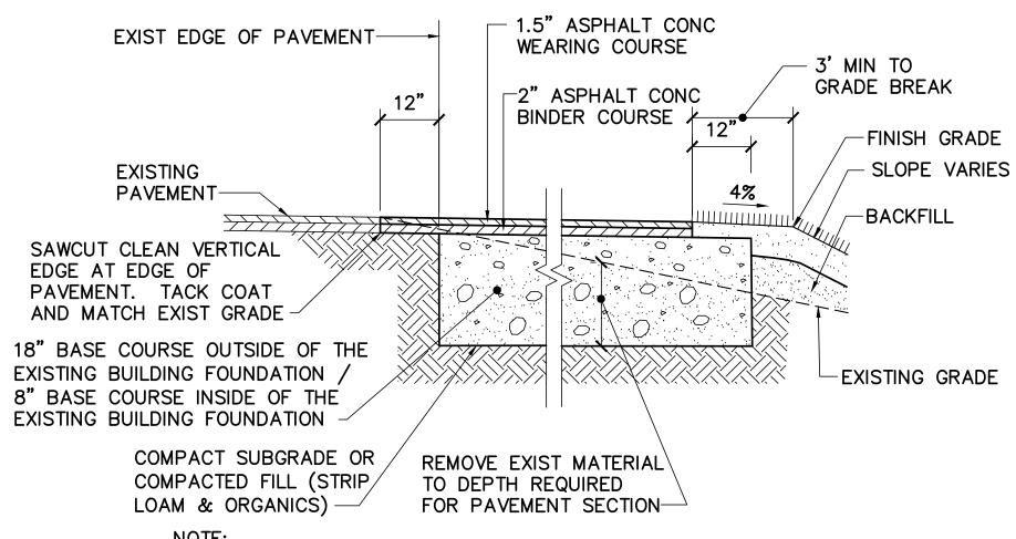
1. AT AREAS WHERE EXISTING PAVEMENT IS REMOVED AND GRAVEL BENEATH PAVEMENT IS NOT REMOVED, DISTURBED OR QUALITY DEGRADED DUE TO CONSTRUCTION ACTIVITIES, FINE GRADE THE PAVEMENT SUGRADE, PROVIDE ADDITIONAL BASE COURSE TO ACHIEVE FINISH GRADES, COMPACT AND PROVIDE WEARING COURSE AND BINDER COURSE.
