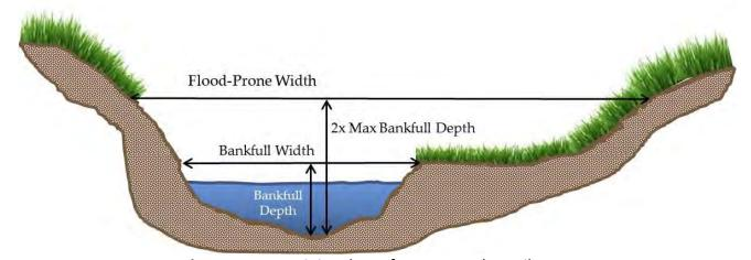
Figure 1: Determining the Reference Reach Attributes.
