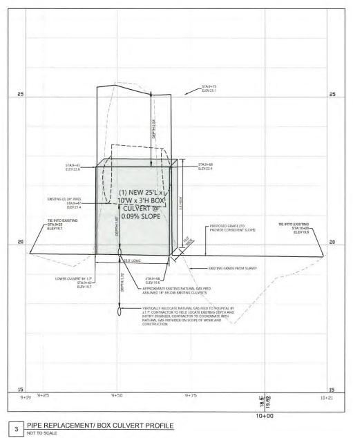
LEGEND EXISTING STAKED WETLAND EXISTING PAVEMENT - GAS - EXISTING GAS MAIN ==== EXISTING STORM DRAIN - PROPOSED CONTOUR PROPOSED CENTERLINE OF DREDGED DRAINAGE CHANNEL PROPOSED 25x7x3' BOX CULVERT
